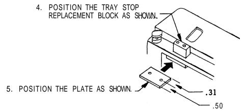
6. SECURE THE BLOCK TO THE PLATE WITH TWO OF THE SCREWS INCLUDED IN THIS KIT.
